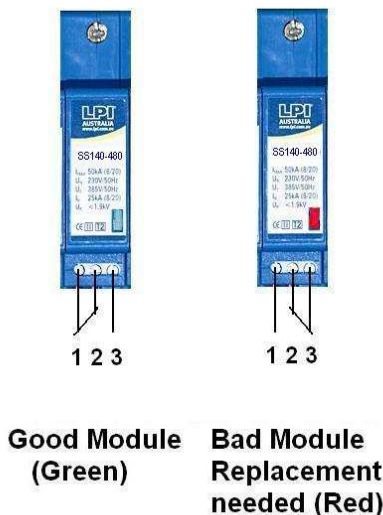
Figure 4. Remote Status Monitoring voltage-free contacts on protection module
